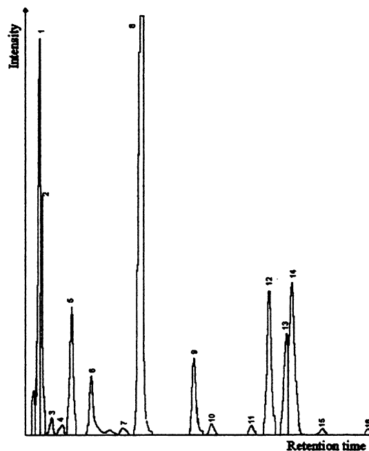
Fig. 5. GC trace of fatty acids of the nutmeg extract obtained with liquid CO 2 at 90 bar and 23.0°C.
